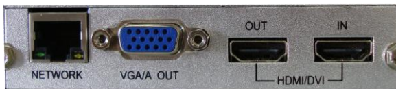
The rear of input module
